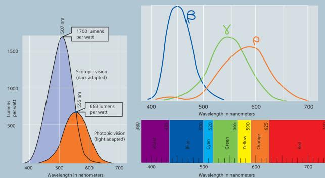
Fig. 3. Sensitivity curves: a) depending on the ambient condition (dark surrounding or not); b) Cones sensitivity curves for red, green and blue cones. c) wavelength scale.
